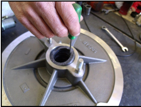
Packing Mount Removed From Pump for Clarity
